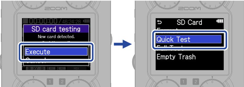
A quick test can check the performance of a microSD card in a short time (about 30 seconds) regardless of its capacity. A full test will check the entire microSD card, so the amount of time required depends on its capacity (about 1.5 hours for 64 GB).
