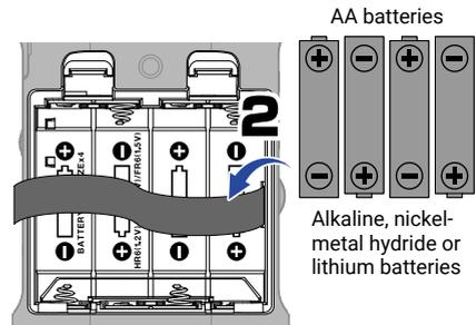
Extend the battery ribbon underneath.
