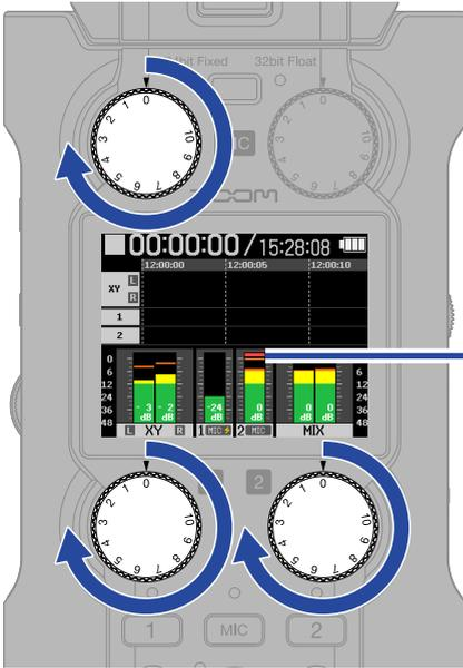
Confirm that the level meters are moving.
