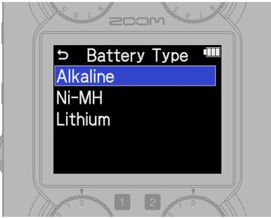
Set the type of battery used correctly so that the amount of remaining battery charge can be shown accurately.
