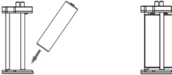
Fig. 2. Inserting batteries into the battery holder
